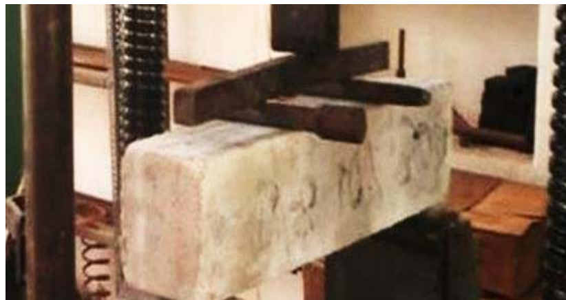
Figure 4.10: Experimental Setup for Flexural Strength.
