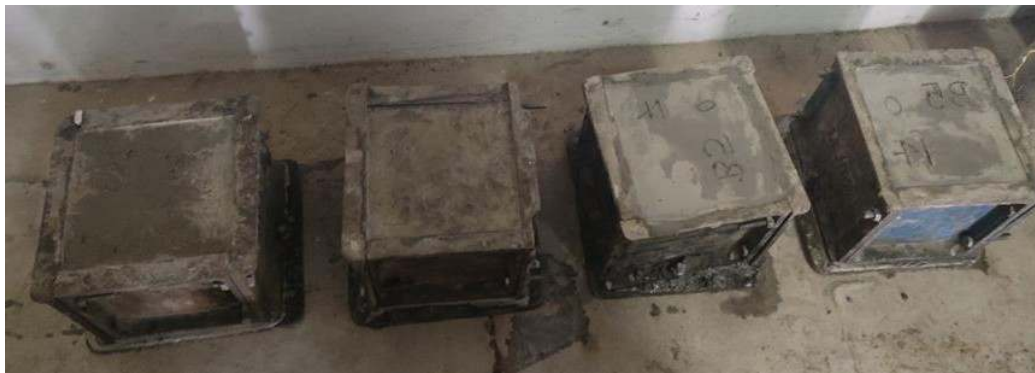
Figure 4.5: Casting of Cubes.
