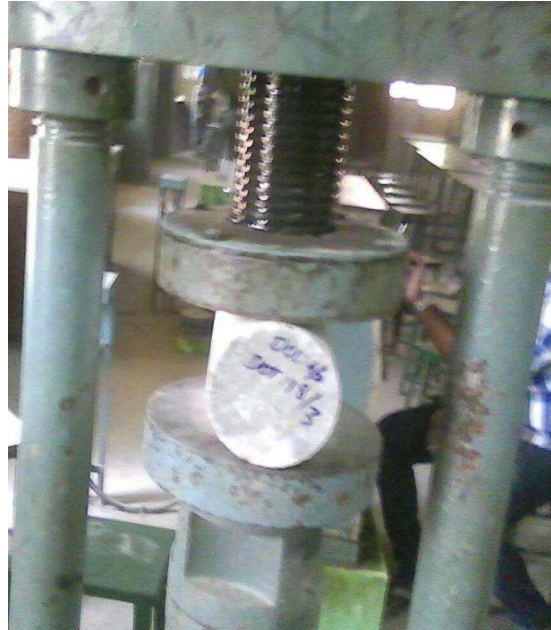
Figure 4.8: Experimental Setup for Split Tensile Strength.
